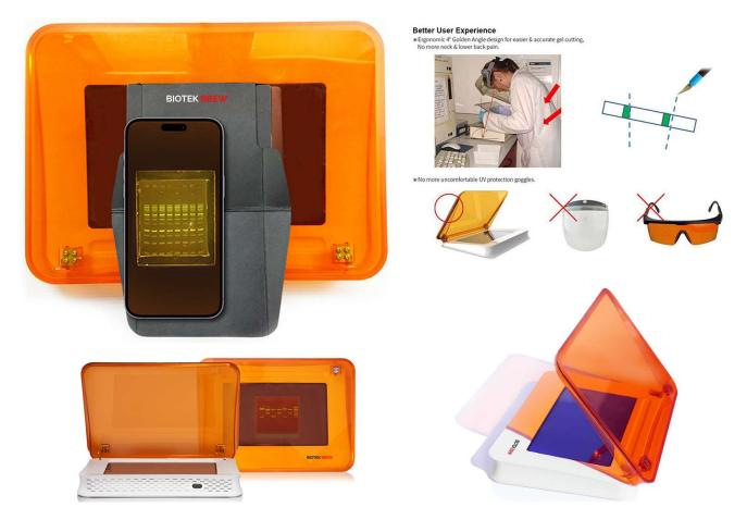
BiotekBrew's LED transilluminator is an extraordinary blue light LED transilluminator for the detection of nucleic acids or protein under non-UV conditions. The wavelength of the special blue LED lights is 470 nm, hence no damage to your nucleic acids or protein. Since UV is not used, there is no need for any special personal eye or skin protection.
